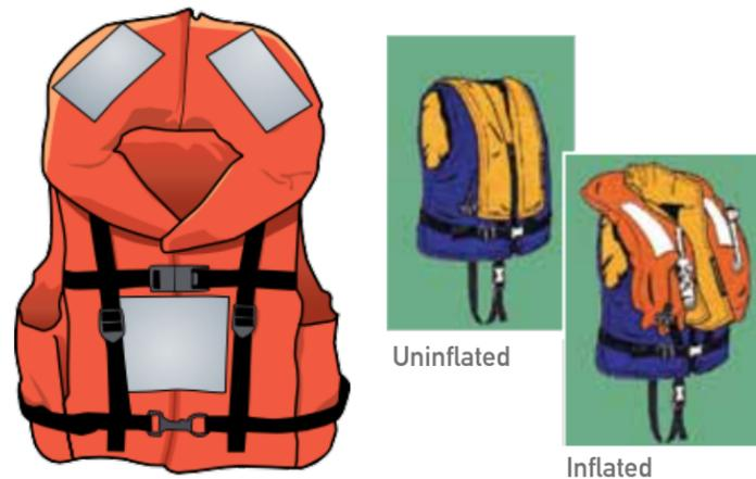
A **Type II, Near-Shore Buoyancy Vest** is intended for calm, inland waters or where there is a good chance of quick rescue. Inherently buoyant life jackets of this type will turn some unconscious wearers to a face-up position in the water, but the turning is not as pronounced as with a Type I. This type of inflatable turns as well as a Type I foam jacket.
